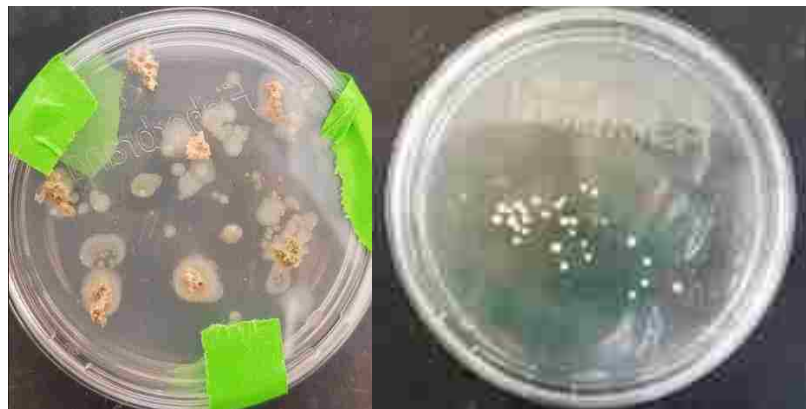
Figure 5-4. Agar-loaded petri dishes to show bacterial presence on the Metamateria (left) and ion exchangers (right) after 24 hours.
